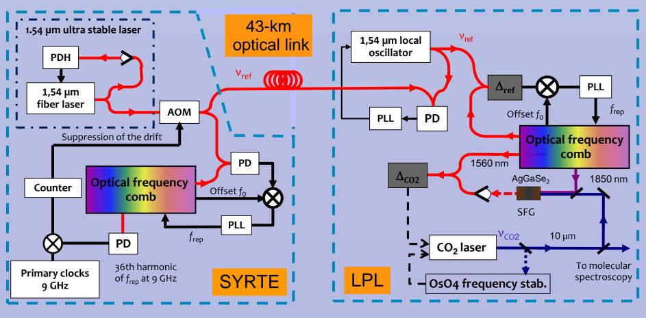
Mid-IR frequency stabilisation onto  $v_{ref}$
